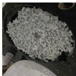
Unprotected and premature transom & outdrive zinc loss
