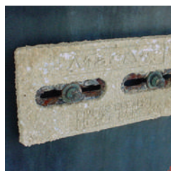
Unprotected and premature transom & outdrive zinc loss
